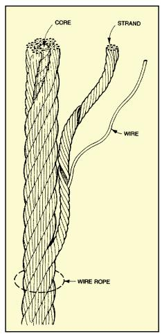
wires is then helically laid together in a uniform geometric pattern to form a strand. This process must be performed with precision and exactness to form a strand of correct size and characteristics. The required number of suitably fabricated strands are laid symmetrically with a definite length of lay around a core, forming the finished wire rope.
