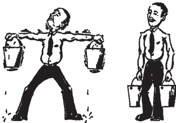
Figure 2A. How do you carry two buckets of water? The above illustration typify the stresses imposed on slings when the legs are attached to the load at various angles.
