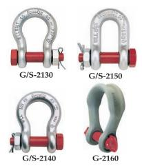
**Bolt-Type Shackles** can be used in any application where round pin or screw pin shackles are used. In addition, they are recommended for permanent or long term installations and where the load may slide on the shackle pin causing the pin to rotate. The bolt-type shackle's secondary securement system, utilizing a nut and cotter, eliminates the requirement to tighten pin before each lift or movement of load.
