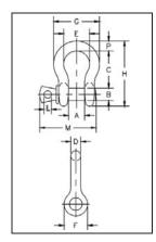
Screw pin anchor shackles meet the performance requirements of Federal Specification RR-C-271D Type IVA, Grade B, Class 2, except for those provisions required of the contractor.
