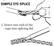
2. Select point where splice is to begin. Insert tapered end of fid between the strands at this point.
