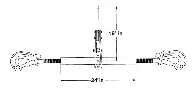
1-3/8" x 24" Stationary (with pelican hook one end and jaw one end) 90,000 Lb. Minimum Breaking Strength
