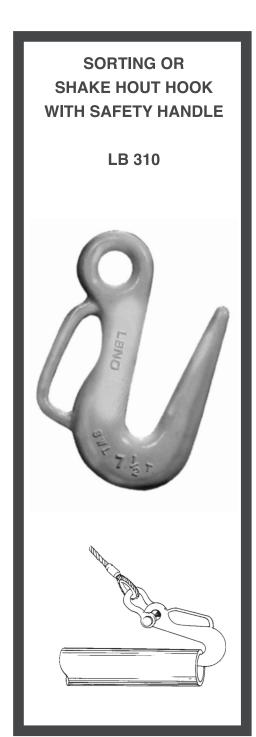
LBNO Sorting Hooks are designed with safety handles to help eliminate the hazard of crushed hands. The generous deep throat dimensions allow for efficient handling of pipe or flat steel plate. The long tapered point allows for easy grabbing of steel beams, links, rings, eye bolts and/or lifting holes.
