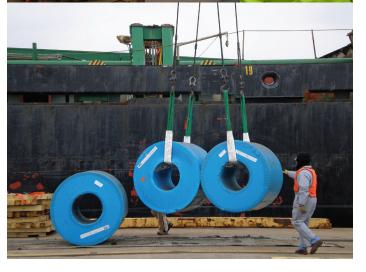
**CORNERMAX® SLEEVE CUT PROTECTION** Damaged or misused protection can result in damage or sling failure. Inspect before each use. Inspect for cuts, tears or damage that may prevent protection of the sling. Ensure protection is the correct size and type to protect the sling. Prevent sleeve and sling from slipping or sliding across load edge. DEATH or INJURY can occur from improper use, maintenance and/or inspection. MAXIMUM LOADING: Do NOT exceed 25,000 lbs. per inch of sling width.
