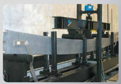
All of our products are tested to ASTM approved plastic lumber specifications. Test details available upon request.
